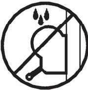
**3.14** - Do not grease or lubricate the winch's braking mechanism. The brake disks have been greased with a special heat and pressure resistant solution. Other products should not be used to avoid negative effects regarding the braking mechanism.
