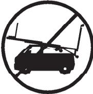
**3.13** - All sections must be lowered first, and the legs placed in its transport position, before transportation.
