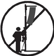
**3.8** - NEVER move the lift whilst it is carrying a load. It is not advisable to carry out any type of horizontal movement even small positional adjustments.
