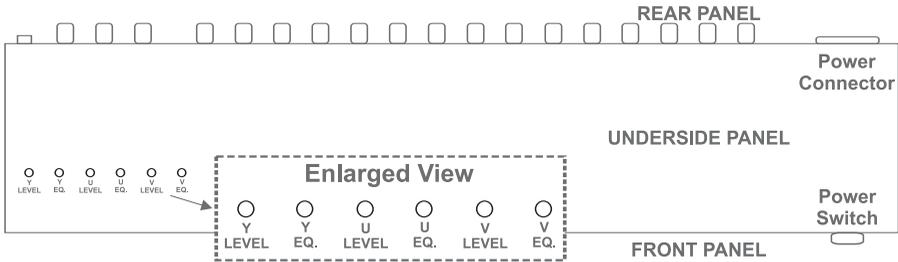
Figure 2: VM-100C Underside Trimmers
